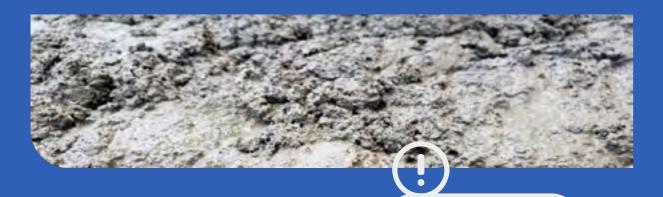
**Ratio of the mass:** 2 tins of sand, 2 tins of gravel and 2 tins of cement. Water for the mixture.
